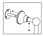
5. Install slide bar into upper escutcheon and trim ring. Install assembly to the upper mounting bracket. Make sure notch in slide bar fits into the pin in the escutcheon. Tighten set screws securely
