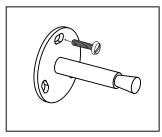
1. Measure complete slide bar from center of the escutcheon to the center of the other escutcheon. Transfer those dimensions to the mounting surface. Attach mounting brackets to the wall. It is highly recommended that the brackets be mounted into a vertical stud.
