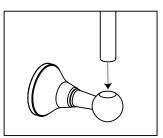
4. Install slide bar into lower escutcheon. Make sure notch in slide bar fits into the pin in the escutcheon. This will prevent any rotation of the slide bar.
