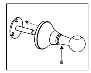
2. Install escutcheon and trim ring to the lower mounting bracket. Use set screw to tighten escutcheon to post of mounting bracket.
